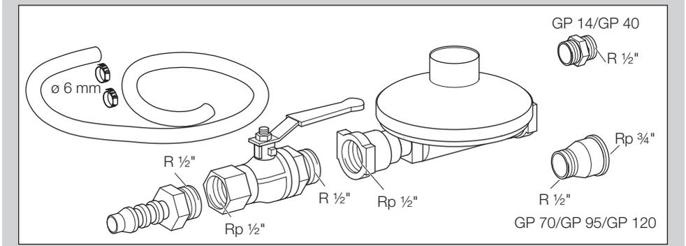
Pressure reducer, manual valve, hose (length = 2 m), 2 hose clamps, R 1/2" double nipple for GP 14/GP 40, R 1/2-Rp 3/4" reducing fitting for GP 70-GP 120, to connect the gas combination control CG to the gas supply, Order No.: N52600025
