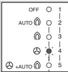
! On burner start-up, the BCU has not detected a flame during the safety time. In the parameter "Number of start-up attempts", it is possible to program up to three start-up attempts. If one of the further start-up attempts is successful, fault signalling stops automatically once the post-purge time has elapsed.
